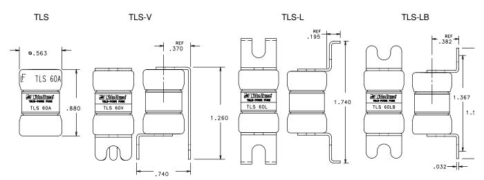
Contact Littelfuse for characteristic curves. Dimensions for reference only. Replaces competitors' TPS and TGS Series.
