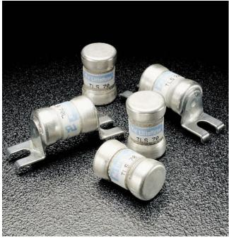
Littelfuse's TLS Series fuses are designed specifically for the protection of telecommunications equipment. TLS fuses have been engineered to operate up to 170 VDC to provide current limiting short circuit protection for cables and components found in the DC power distribution circuits of telecommunications systems. The TLS' compact design provides superior protection and high power density in an extremely compact package.
