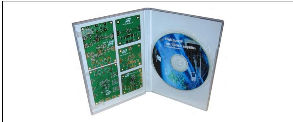
Figure 29. Evaluation kit for high-speed op-amps
