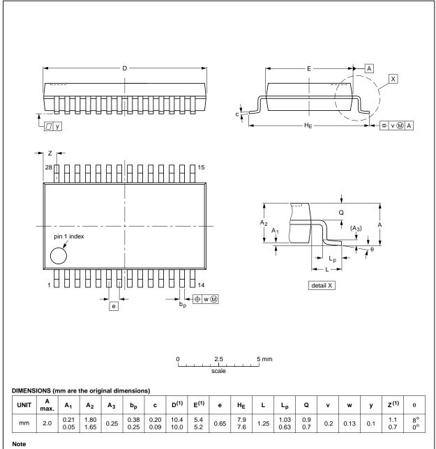
1. Plastic or metal protrusions of 0.20 mm maximum per side are not included.
