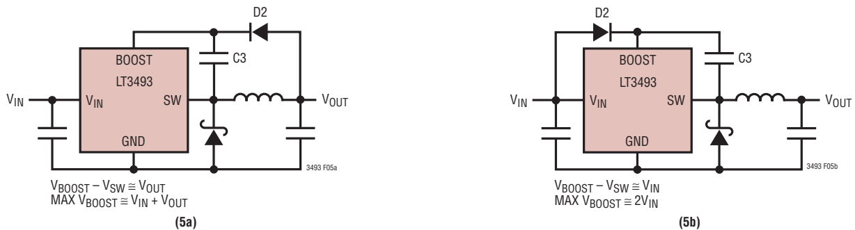
Figure 5. Two Circuits for Generating the Boost Voltage
