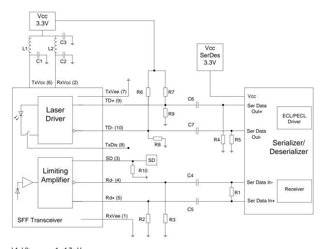
$\begin{array}{lll} \text{L1, L2:} & 1...4.7 \ \mu\text{H} \\ \text{C1, C2, C3:} & 4.7...10 \ \mu\text{F} \\ \text{C4, C5, C6, C7:} \ 100 \ n\text{F} \\ \text{R1:} & 100 \ \text{Ohms} \\ \text{R2, R3:} & 150 \ \text{Ohms} \end{array}$
