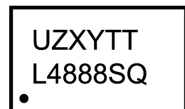
Top View U = Fab Code Z = Assembly Plant Code XY = Date Code TT = Die Traceability
