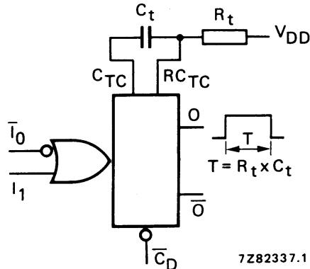
Fig.4 Connection of the external timing components  $R_t$  and  $C_t$ .
