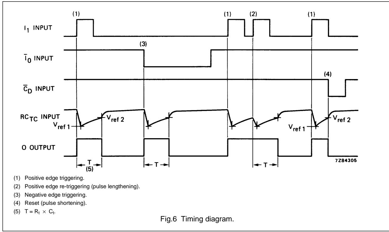
Fig.6 Timing diagram.
