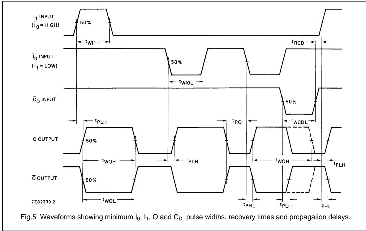
Fig.5 Waveforms showing minimum  $\bar{I}_0$ ,  $I_1$ , O and  $\bar{C}_D$  pulse widths, recovery times and propagation delays.
