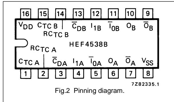
Fig.2 Pinning diagram.
