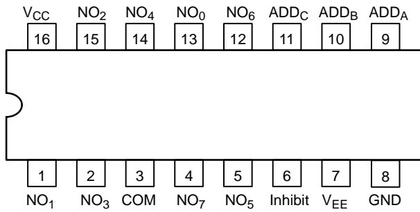
Figure 1. Pin Connection (Top View)
