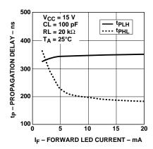
Figure 12. Propagation Delay vs. Input Current.
