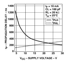
Figure 11. Propagation Delay vs. Supply Voltage.
