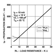
Figure 9. Propagation Delay vs. Load Resistance.
