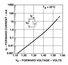
Figure 4. Input Current vs. Forward Voltage.
