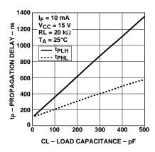
Figure 10. Propagation Delay vs. Load Capacitance.
