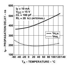
Figure 8. Propagation Delay with Internal 20  $k\Omega\,RL$  vs. Temperature.
