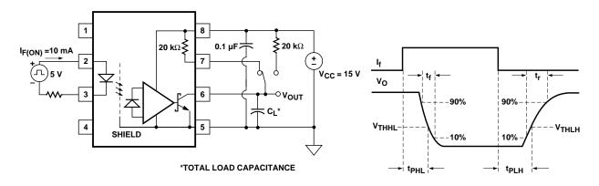
Figure 5. Propagation Delay Test Circuit.
