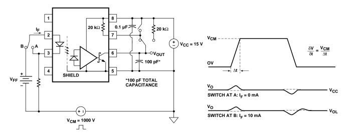
Figure 6. CMR Test Circuit. Typical CMR Waveform.
