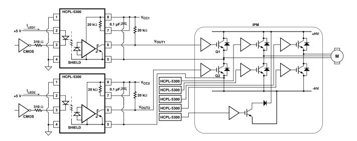
Figure 22. Typical Application Circuit.
