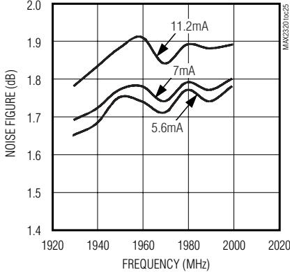
**PCS-BAND HGLL LNA NOISE FIGURE vs. FREQUENCY**
