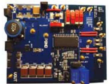
75mm x 58mm, Single Layer PCB for a 45W backlight
