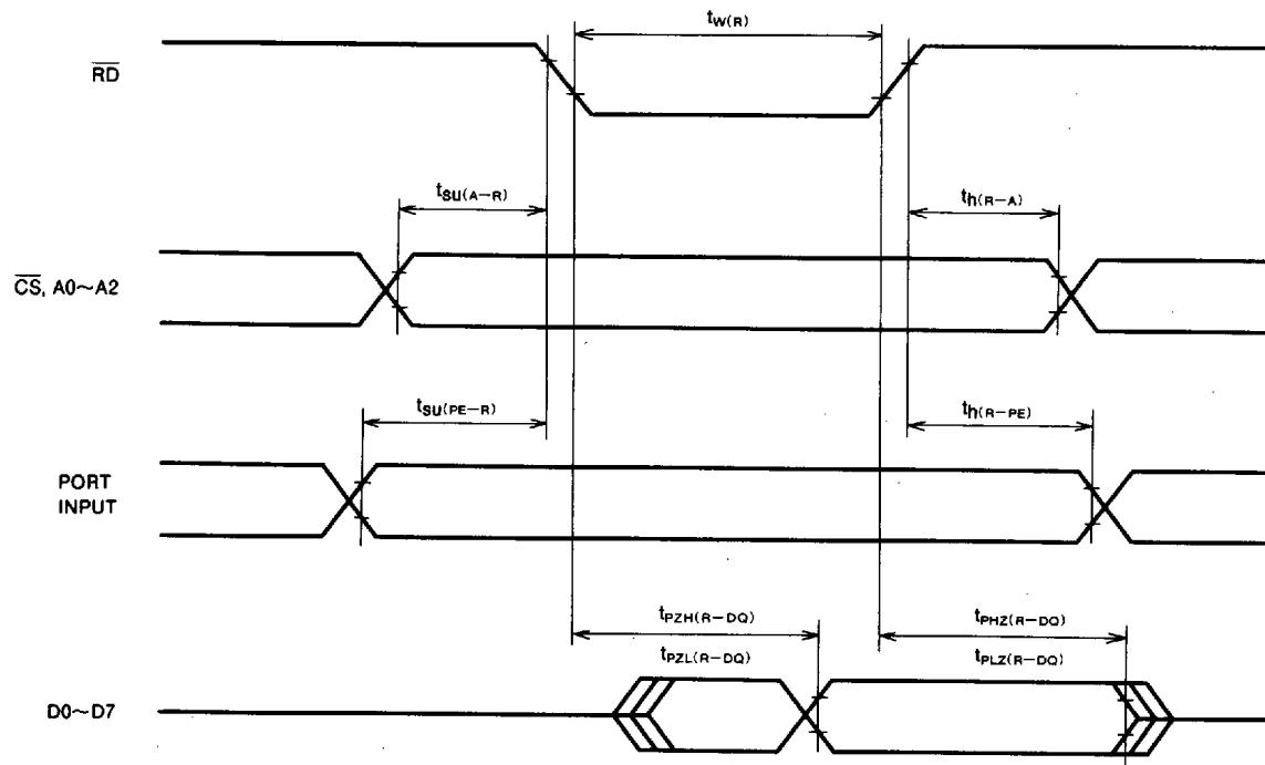
Write operation timing (includes control register write)
