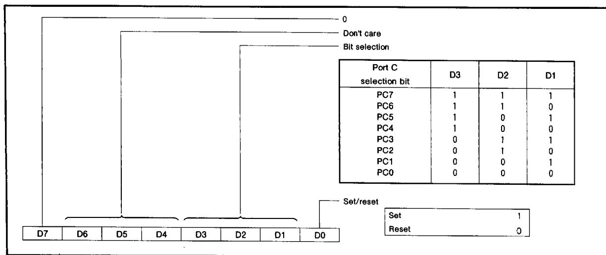
Fig. 2 Port C bit set/reset control word
