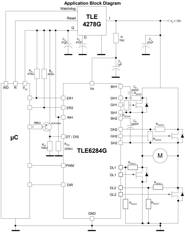
This application block diagram shows one of the possibilities to use this Driver IC. The voltage divider networks accross the 4 MOSFETs (resistors  $R_{SCDxx}$ ) allow to increase the current limit threshold for Short Circuit protection. The  $R_{SCDLx}$  resistors also provide a charge path for the bootstrap capacitors. If  $R_{SCDLx}$  resistors are not used in the application, a 12k Ohm resistor should be introduced between SH1 to GND and SH2 to GND.
