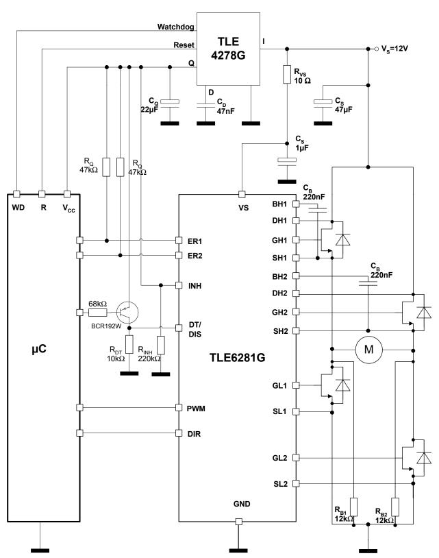
This example application circuit shows one possibility to use this Driver IC.
