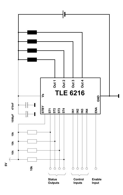
The blocking capacitor C is recommended to avoid critical negative voltage spikes on VS in case of battery interruption during OFF-commutation.
