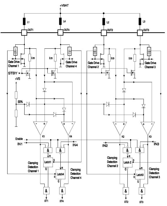
**Block Diagram of Open Load Detection**
