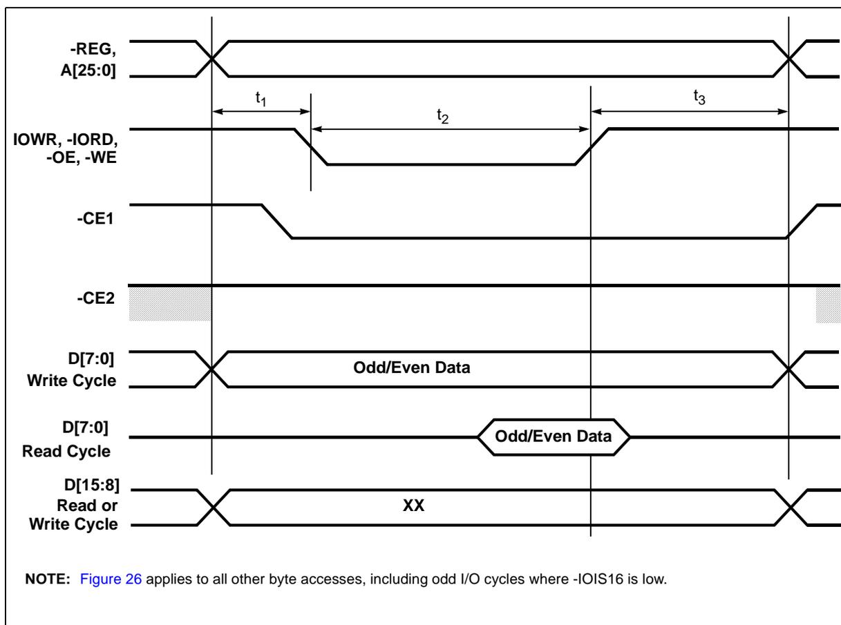
**Table 35. 16-Bit System to 8-Bit I/O Card: Odd Byte Timing**
