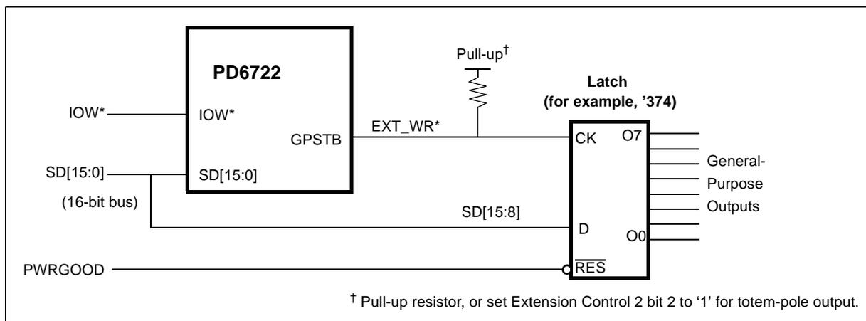
In this mode, **Extension Control 2** register bit 4 is set to '1' enabling the GPSTB pin to function as a write strobe. Writes to the respective extended index 0Ah cause the respective GPSTB to go active (low) for the duration of the system's IOW\* pulse.
