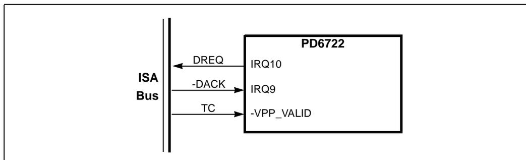
Terminal counts are passed through to the card from the PD6722 -VPP\_VALID pin when bit 6 of the **Misc Control 2** register is '1'. For a DMA write process, the last-cycle terminal count condition is indicated by -OE being active-low during a card DMA data read cycle. For a DMA read process, terminal count is indicated by -WE being active-low during the last card cycle.
