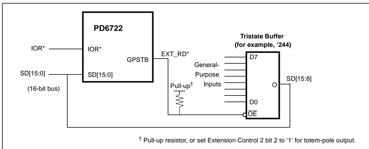
In this mode, **Extension Control 2** register bit 3 is set to '1', enabling the respective GPSTB pin to function as a read strobe. Reads from the corresponding extended index 0Ah cause GPSTB to go active (default active level is low) for the duration of the system's IOR\* pulse.
