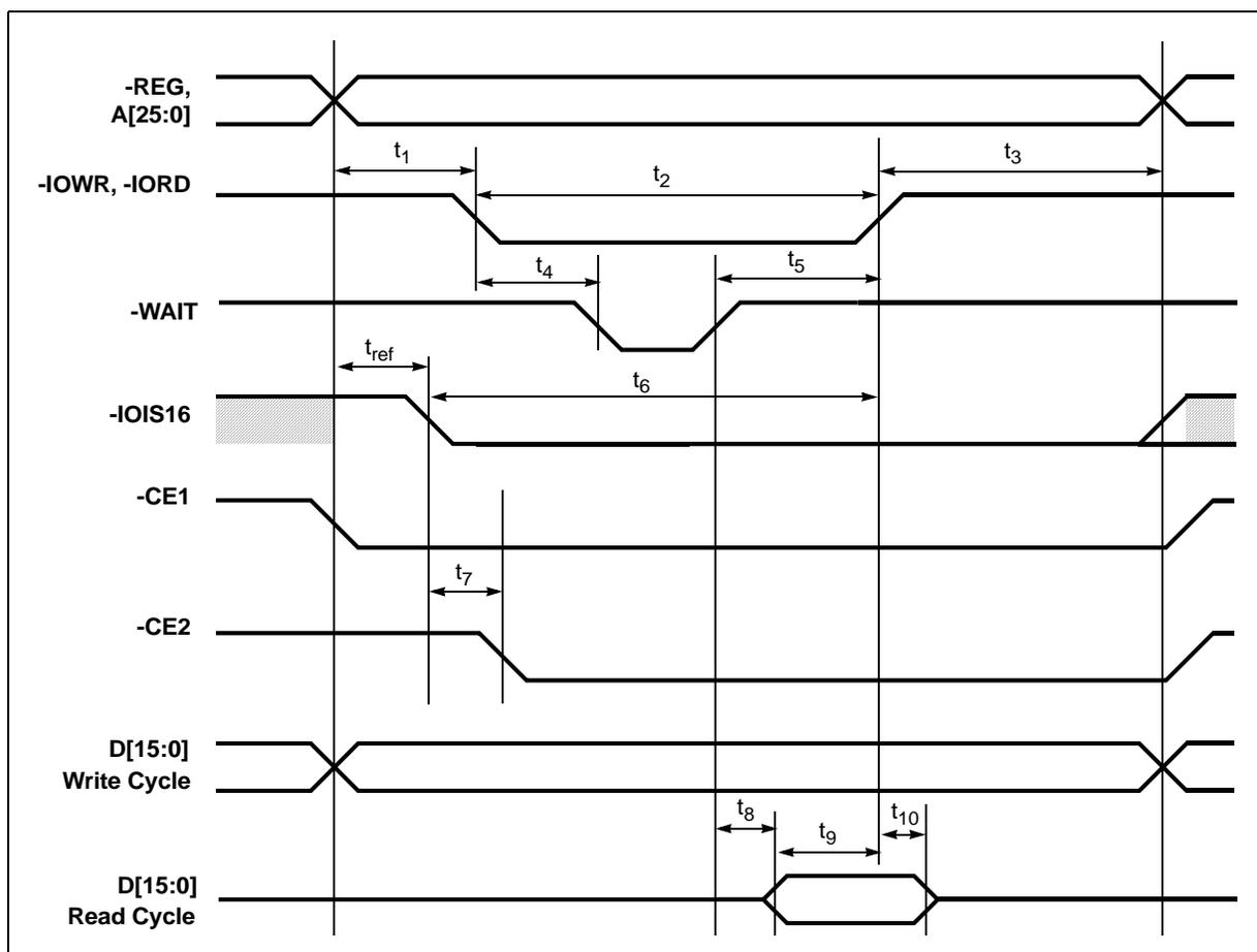
**Table 33. PC Card Read/Write Timing when System Is 8-Bit**
