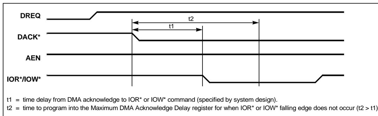
The maximum DMA acknowledge delay (t2 as shown in Figure 12) should be programmed to a time greater than the maximum time required from the system’s issuance of a DMA acknowledge to its issuance of a DMA read or write cycle (t1 as shown in Figure 12). The t1 time is indicated in the specifications for the systems DMA cycle timing.
