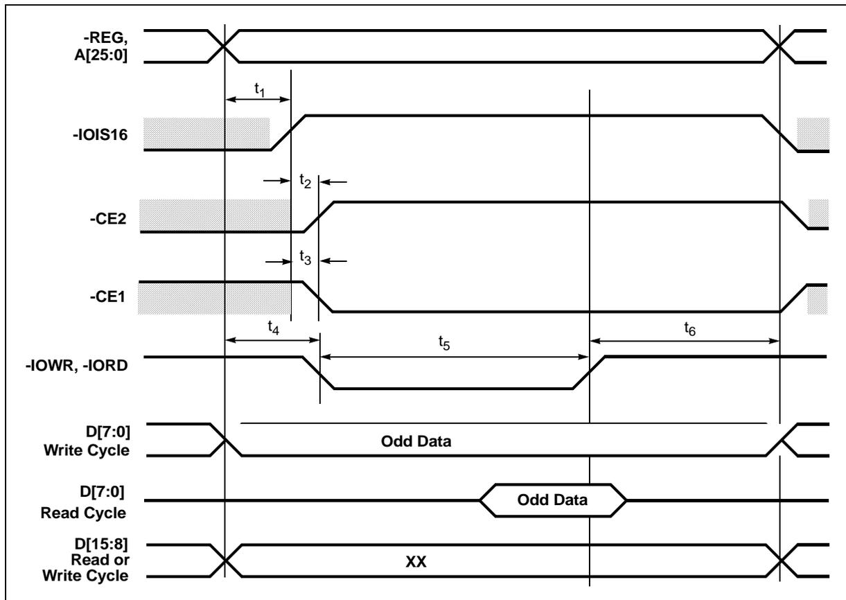
Table 36. DMA Read Cycle Timing (PD6722 only) (Sheet 1 of 2)
