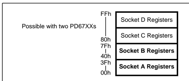
When viewed as a 8-bit value, the contents of the **Index** register completely specify a single internal-register byte. For example, when the value of this register is in the range 00h–3Fh, a Socket A register is selected (Socket Index bit is ‘0’), and when the value of this register is in the range 40h–7Fh, a Socket B register is selected (Socket Index bit is ‘1’). This register only reads back for Device 0. Device 1 will read back only the upper data byte when 16-bit reads occur at 3E0h.
