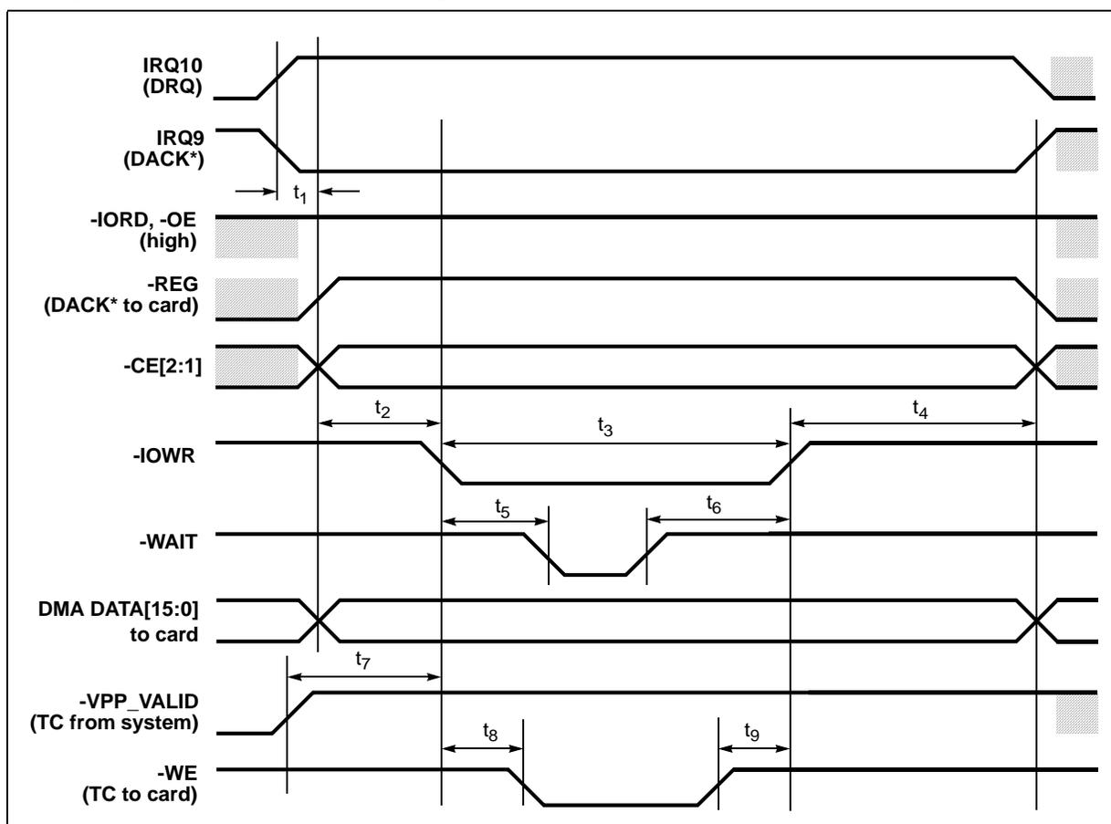
Table 37. DMA Write Cycle Timing (PD6722 only)
