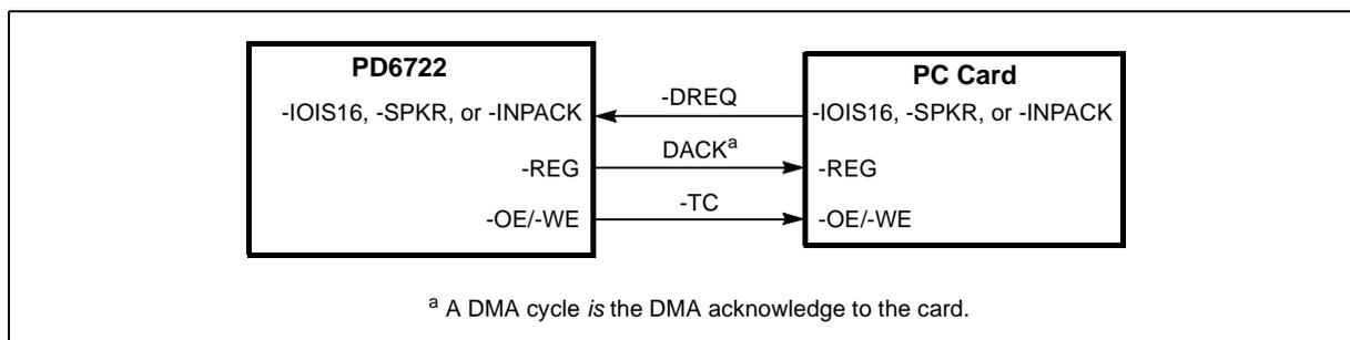
Notice that the DMA acknowledge to the card as -REG high is only active during the actual DMA read or write card cycle. This means there is no mechanism to deassert DACK to the card: The card must understand that receiving the first DMA cycle *is* its DMA acknowledgment.
