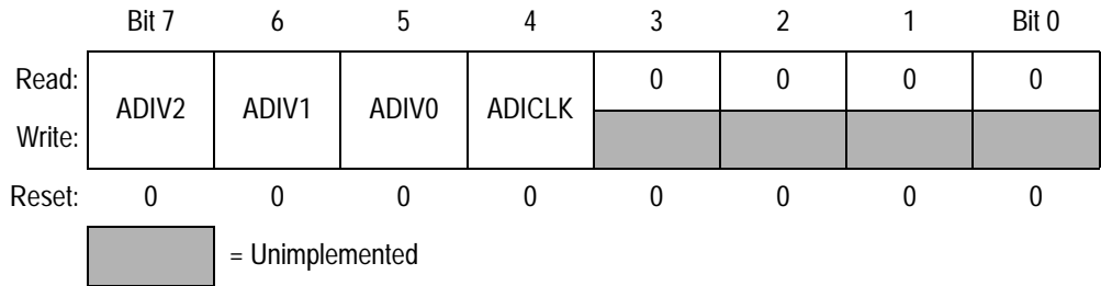
Figure 5-4. ADC Clock Register (ADCLK)
