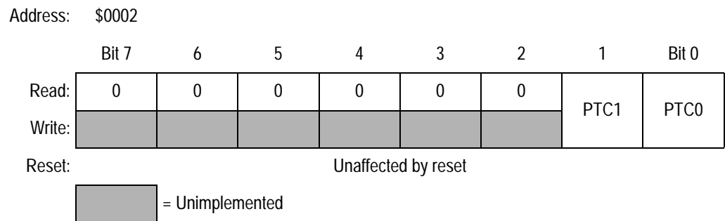
Figure 16-9. Port C Data Register (PTC)
