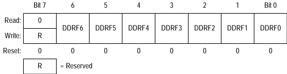
Figure 20-18. Data Direction Register F (DDRF)
