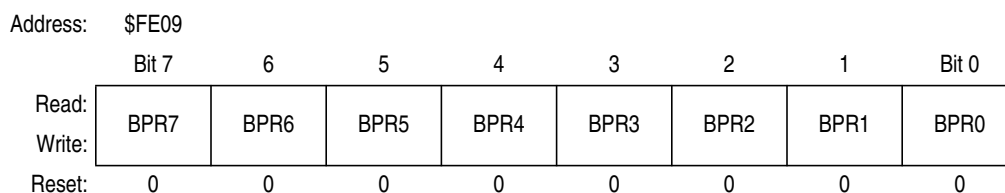
Figure 2-5. FLASH Block Protect Register (FLBPR)
