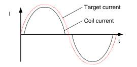
Coil current does not have optimum shape
