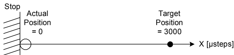
Figure 19: Positioning Example: Situation after reference search
