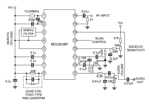
In the above typical application, the audio signal is recovered using a conventional quadrature FM detector. The absence of an input signal is indicated by the presence of noise above the desired audio frequencies. This "noise band: is monitored by an active filter and a detector. A squelch trigger circuit indicates the presence of noise (or a tone) by an output which can be used to control scanning. At the same time, an internal switch is operated which can be used to mute the audio.
