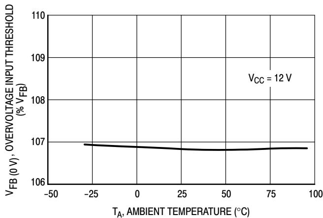
**Figure 2. Overvoltage Comparator Input Threshold versus Temperature**
