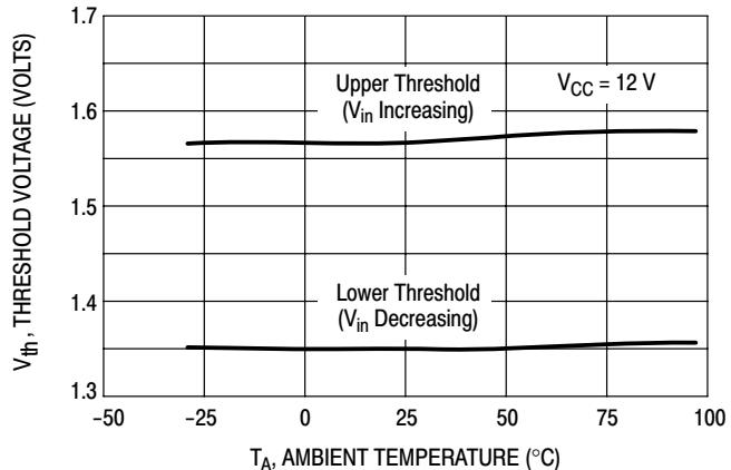
**Figure 7. Zero Current Detector Input Threshold versus Temperature**
