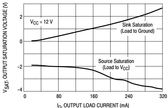
**Figure 6. Output Saturation Voltage versus Load Current**
