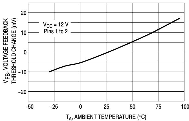
**Figure 4. Voltage Feedback Input Threshold Change versus Temperature**
