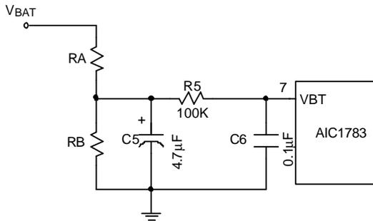
**FIG. 1 Battery Voltage Divider**
