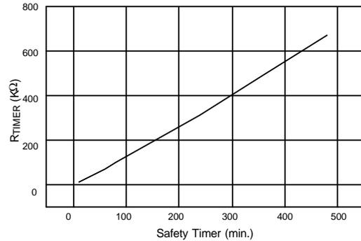
**Fig. 3 Safety Timer vs.  $R_{TIMER}$**
