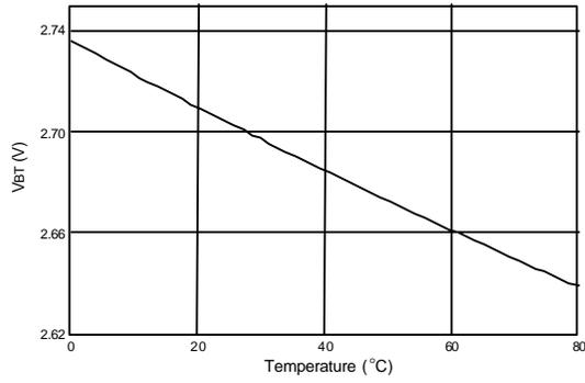
$V_{BT(Low)}$  Limits vs Temperature (After Initial Timer)
