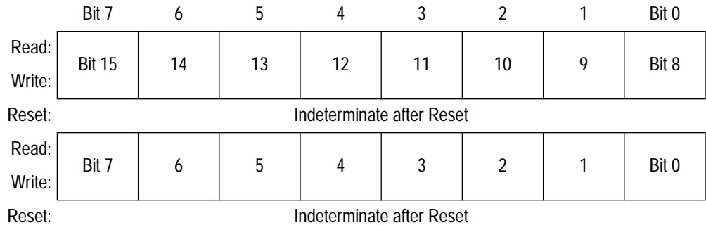
Figure 13. TIM Channel Registers (TCH0H/L–TCH3H/L)
