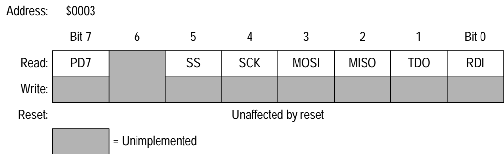
Figure 7-10. Port D Fixed Input Register (PORTD)
