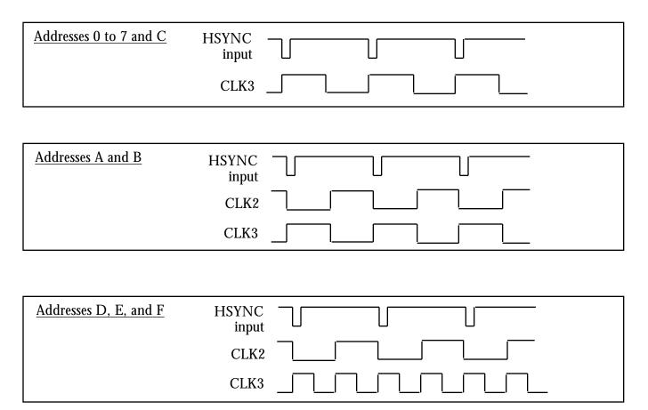
The recovered clocks are triggered by the falling edge of HSYNC and are delayed by about 100ns.
