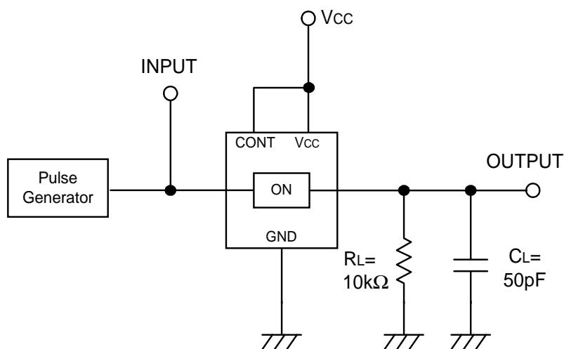
Note: open output when measuring supply current
