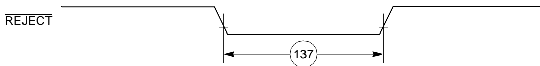
Figure 63. CAM Interface REJECT Timing Diagram
