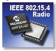
The ZigBee protocol is an industry standard protocol for wireless networking. Specifically designed for low cost and relatively low bandwidth automation applications it allows the quick deployment of several networking flexible topologies, including star, cluster and mesh.
