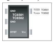
Low cost temperature sensing devices such as the TC6501 and TC6502 (offered in SOT-23 packages) can be conveniently placed near power LED(s) to obtain a more accurate temperature monitoring and provide a logic output fault signal.
