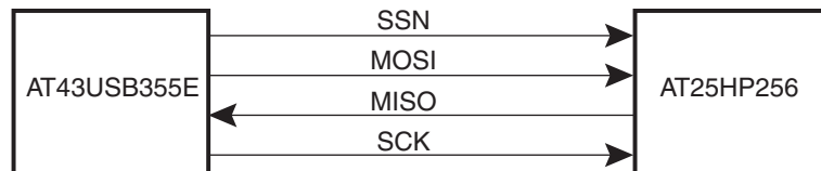
Figure 4. AT43USB355E Read Sequence
