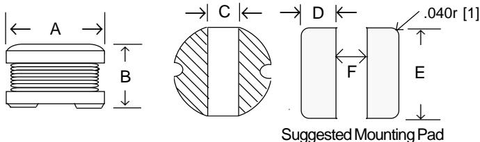
Series PIC inductors were developed to provide high current capability in an economical surface mount design. The cylindrical geometry enables a wide range of values with excellent high frequency performance. Construction is wirewound and utilizes a ferrite core. Units are marked with inductance value. Applications include noise filtering, DC/DC converters, telecom, power supplies, switching regulators, etc. Custom models available.
