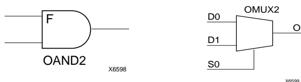
Figure 20: AND & MUX Symbols in XC4000X IOB
