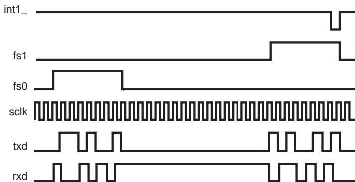
Figure 21. CODEC Interface Timing (8-Bit Mode)
