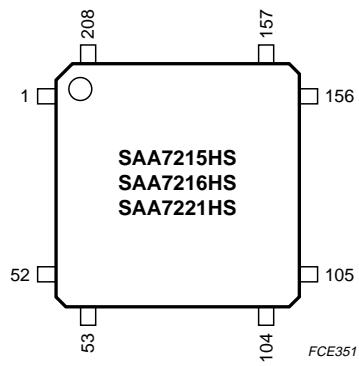
Fig.4 Pin configuration.
