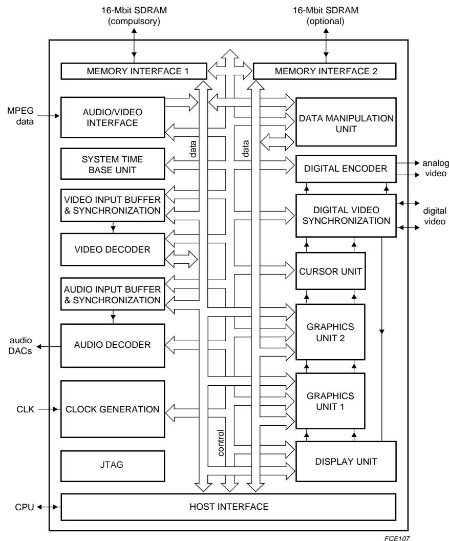
Fig.1 Block diagram.
