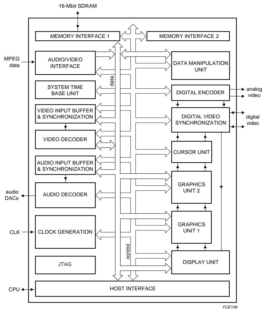
Fig.2 Block diagram with preferred use in 16-Mbit configuration.
