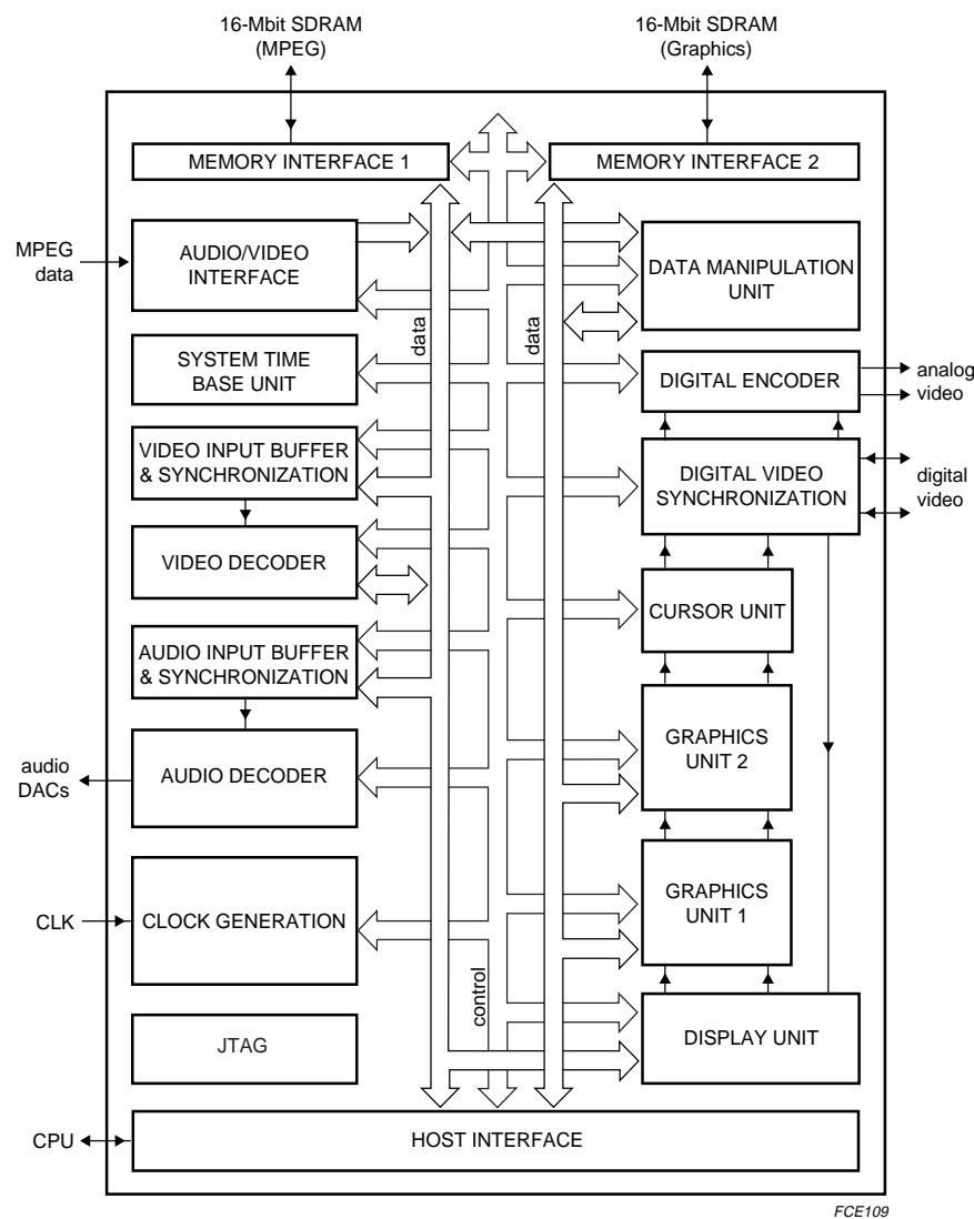
Fig.3 Block diagram with preferred use in 32-Mbit configuration.
