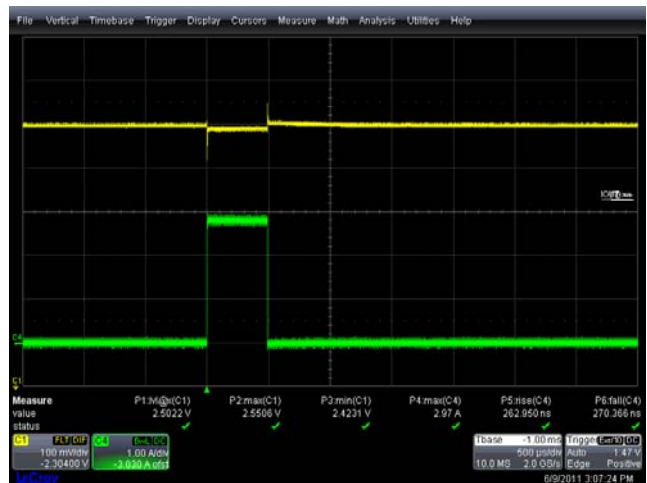
FIGURE 20. TRANSIENT LOAD RESPONSE, V_{IN} = 3.3V , V_{OUT} = 2.5V , C_{OUT} = 220\mu F , 25m \Omega
