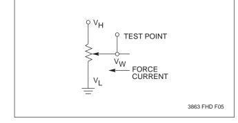
Notes: (1) Absolute Linearity is utilized to determine actual wiper voltage versus expected voltage
