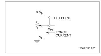
Notes: (1) Absolute Linearity is utilized to determine actual wiper voltage versus expected voltage
