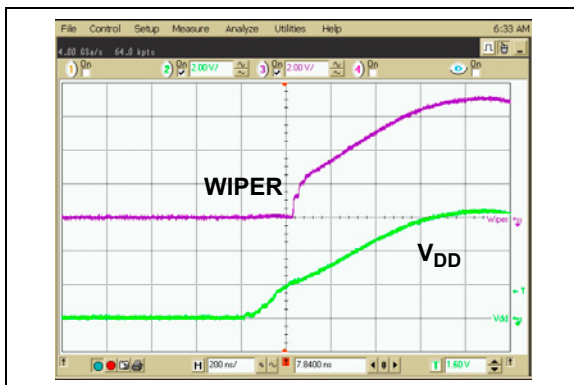
FIGURE 2-45: 50\text{ k}\Omega – Power-Up Wiper Response Time.
