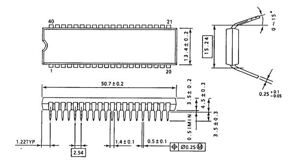
Note: Package width and length do not include mold protrusion, allowable mold protrusion is 0.15mm.
