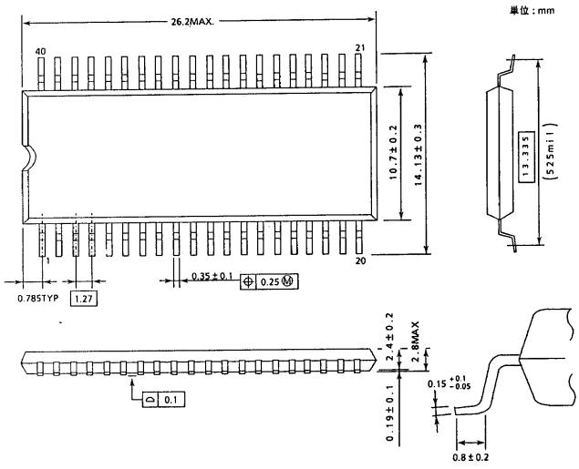
Note: Package width and length do not include mold protrusion, allowable mold protrusion is 0.15mm.
