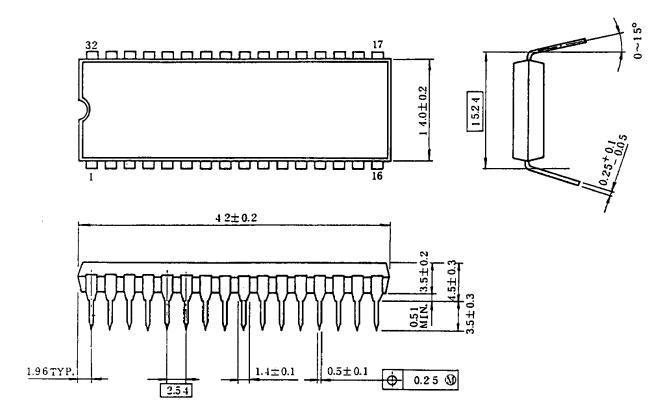
Note: Package width and length do not include mold protrusion, allowable mold protrusion is 0.15mm.
