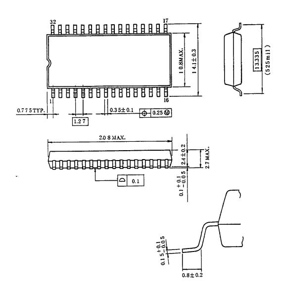
Note: Package width and length do not include mold protrusion, allowable mold protrusion is 0.15mm.
