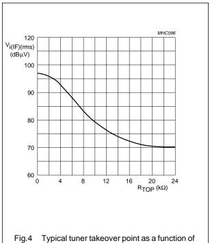
Fig. 4 Typical tuner takeover point as a function of  $$R_{\mbox{\scriptsize TOP}}$.$
