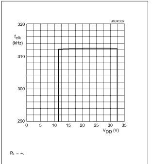
Fig.27 Clock frequency as a function of supply voltage.
