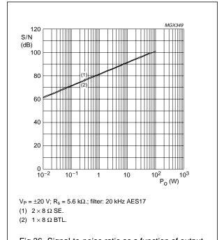
Fig.36 Signal-to-noise ratio as a function of output power.
