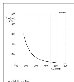
Fig.34 PWM residual voltage as a function of clock frequency.
