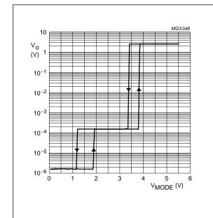
Fig.36 Output voltage as a function of mode selection voltage.
