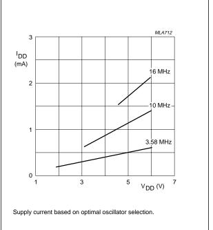
Fig.4 Typical operating supply current ( $I_{DD}$ ) as a function of operating supply voltage ( $V_{DD}$ ).
