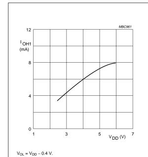
Fig.13 Typical HIGH level push-pull output source current (I<sub>OH1</sub>) as a function of operating supply voltage (V<sub>DD</sub>).
