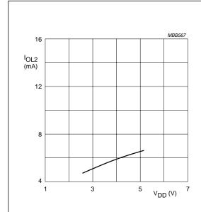
Fig.11 Typical LOW level output sink current for SDA/P2.3 or SCLK ( $I_{OL2}$ ) as a function of operating supply voltage ( $V_{DD}$ ).
