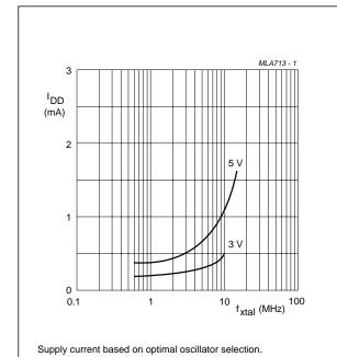
Fig.5 Typical operating supply current ( $I_{DD}$ ) as a function of clock frequency ( $f_{xtal}$ ).
