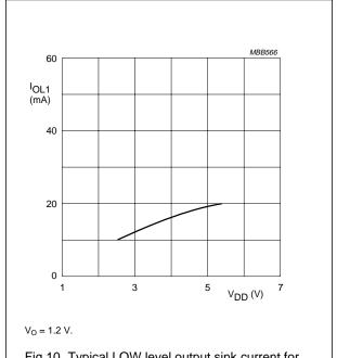
Fig.10 Typical LOW level output sink current for Port 1 (I<sub>OL1</sub>) as a function of operating supply voltage (V<sub>DD</sub>).
