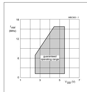
Fig.3 Maximum clock frequency as a function of operating supply voltage (V<sub>DD</sub>).
