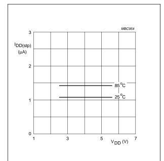
Fig.8 Typical supply current in Stop mode  $(I_{\text{DD(stp)}})$  as a function of operating supply voltage (V<sub>DD</sub>).
