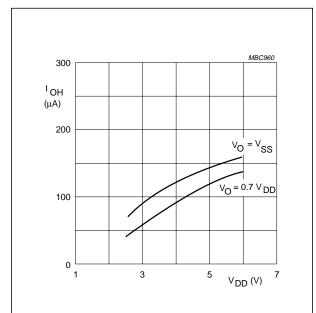
Fig.12 Typical HIGH level pull-up output source current ( $I_{OH}$ ) as a function of operating supply voltage ( $V_{DD}$ ).
