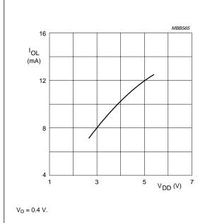
Typical LOW level output sink current (I<sub>OL</sub>) as a function of operating supply voltage  $(V_{DD}).$
