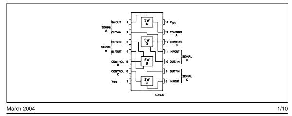
and n device in a given switch are biased ON or OFF simultaneously by the control signal. As shown in schematic diagram, the well of the n-channel device on each switch is either tied to the input when the switch is ON or to  $V_{SS}$  when the switch is OFF. This configuration eliminates the variation of the switch-transistor threshold voltage with input signal, and thus keeps the ON resistance low over the full operating signal range. The advantages over single channel switches
