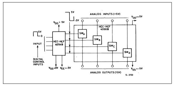
**TYPICAL APPLICATIONS** (BIDIRECTIONAL SIGNAL TRANSMISSION VIA DIGITAL CONTROL LOGIC)
