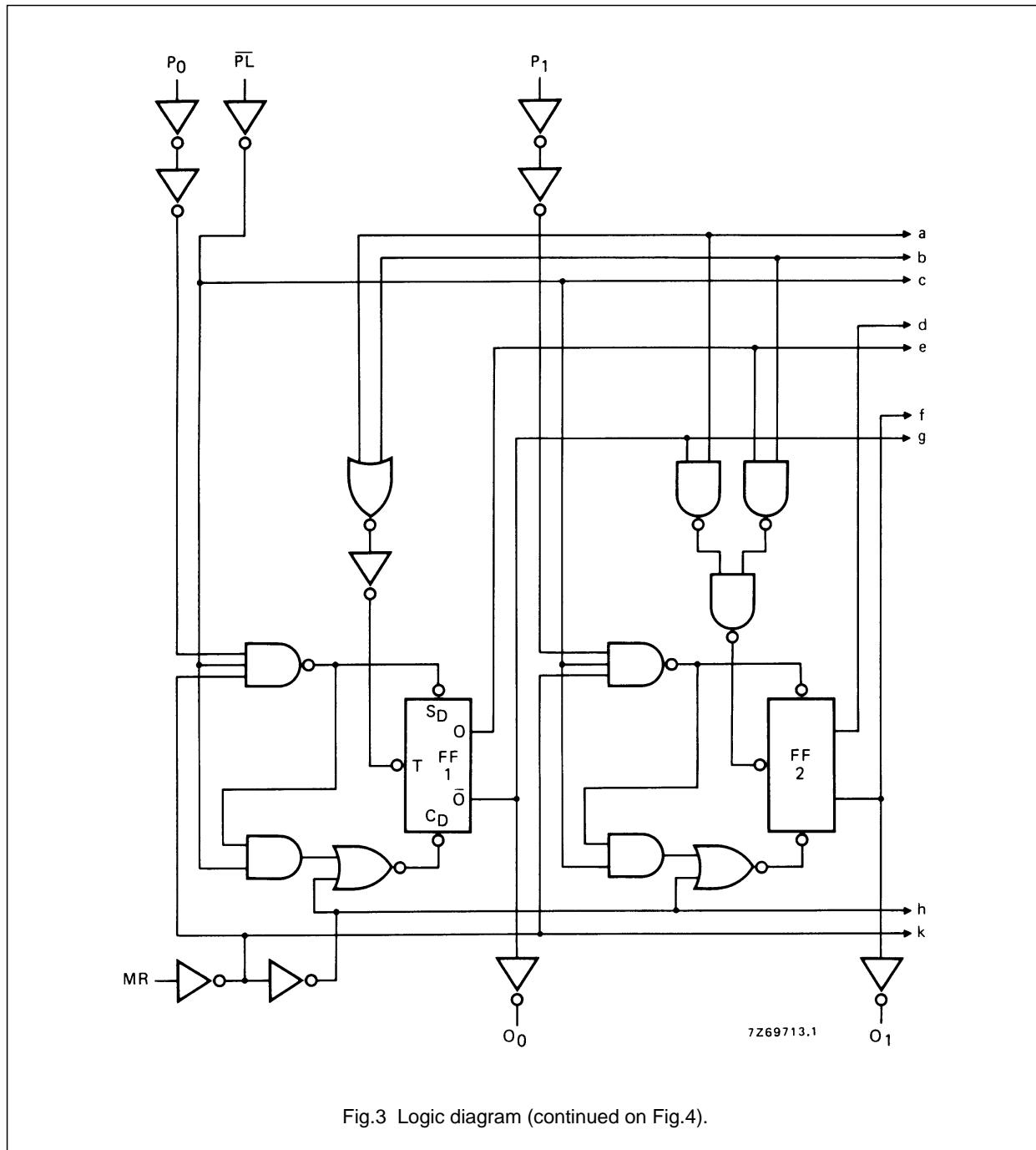
Fig.3 Logic diagram (continued on Fig.4).
