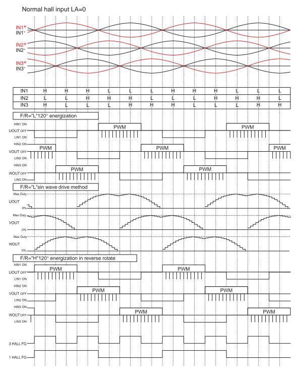
The energization is switched to 120° when 3 Hall FG frequency is 6.1Hz (TYP) or lower A direction of rotation is detected from Hall signal according to F/R pin input
