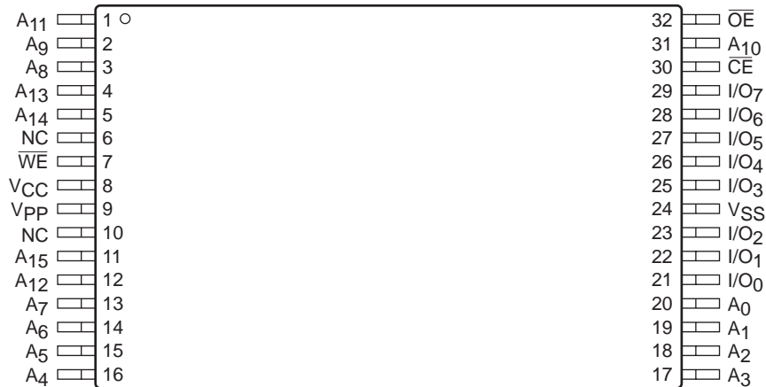
TSOP Package (Standard Pinout 8mm x 20mm) (T)
