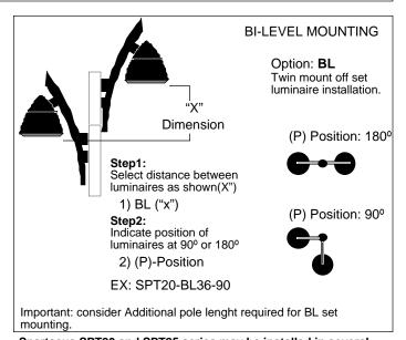
Spartacus SPT20 and SPT25 series may be installed in several positions along the pole. Please provide information with desired position as shown above.
