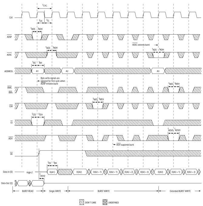
Note: 23. Full width Write can be initiated by either  $\overline{GW}$  LOW; or by  $\overline{GW}$  HIGH,  $\overline{BWE}$  LOW and  $\overline{BW}_X$  LOW.
